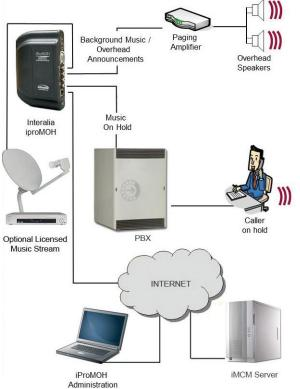
Figure 3 – Typical Connection Diagram prior to the iProMOH calling in.
