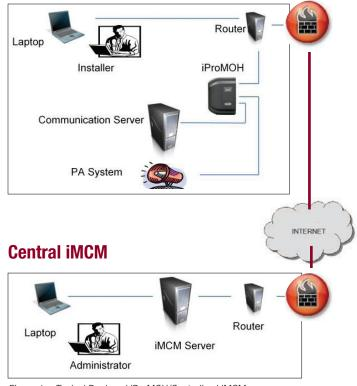
Figure 1 – Typical Deployed iProMOH/Centralized iMCM Network Layout
